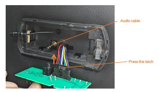
**Step 4**: Connect the new board then proceed with the reassembly (steps 3 to 1).
