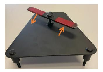
**Step 4**: Install the tool in the same holes that keep the seat cushion in place then hand-tighten the same three (3) nuts that hold the cushion to the disassembly tool:
