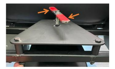
**Step 6:** Hold the circular base with the foot then rotate the Haptic Module until reaching the stopper. Continue to rotate the module than pull it to remove it:
