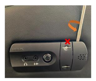
**Step 2:** Remove the microphone from its socket. Using a flat screwdriver, gently push the four (4) tabs (one at the time) to detach the board from the moulding plate:
