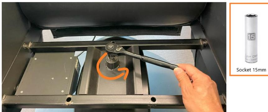
**STEP 3:** Using the D-BOX disassembly tool, turn counterclockwise the red handle to reach its maximum:
