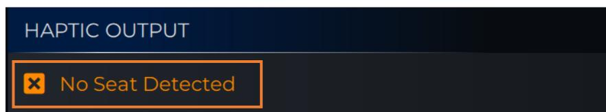
**STEP 1:** Verify that all cables are firmly plugged in to the corresponding ports (**see section 5**).
