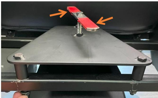
**STEP 6:** Hold the circular base with the foot then rotate the Haptic Module until reaching the stopper. Continue to rotate the module, then pull it to remove it:
