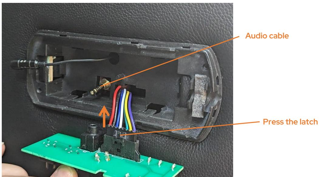
**STEP 4:** Connect the new board then proceed with the reassembly (steps 3 to 1).
