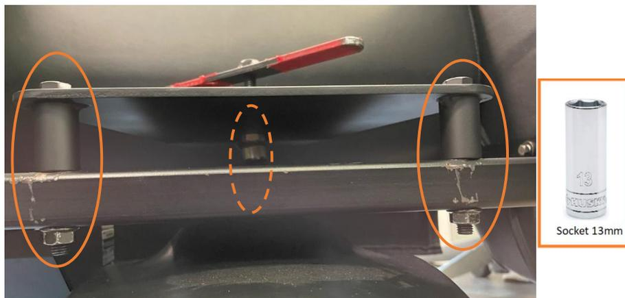
**STEP 5:** Turn clockwise the red handle until the seat frame pops out from the Haptic Module:
