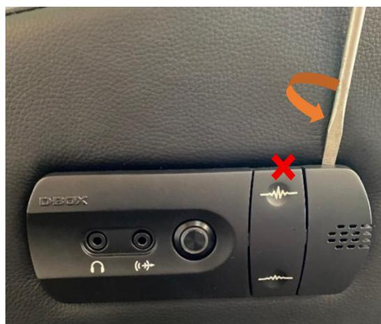
**STEP 2:** Remove the microphone from its socket. Using a flat screwdriver, gently push the four (4) tabs (one at the time) to detach the board from the molding plate:
