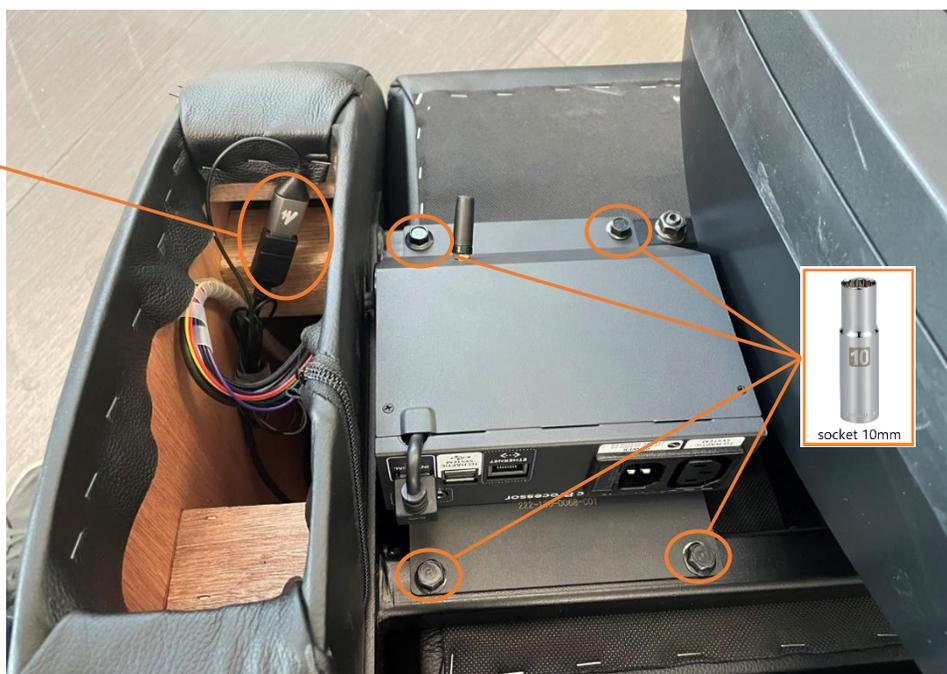
**STEP 3:** Remove the Haptic Processor with its cable harness then install the new one:
