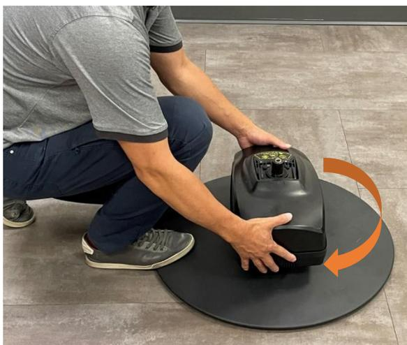
**STEP 7:** Insert the new Haptic Module into the hole of the circular base:
