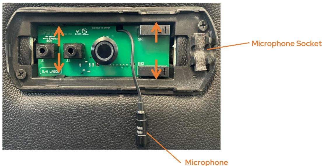
**STEP 3:** Disconnect the black connector from the board by pressing the latch. Disconnect the audio cable then remove the electronic board:
