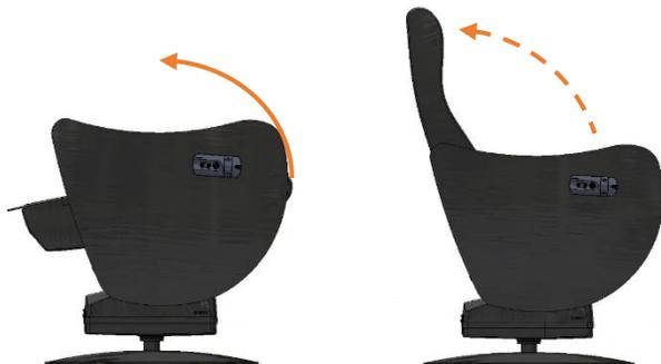
**STEP 4:** Secure the backrest by tightening both screws located at the rear bottom of the seat using a 13mm wrench:
