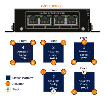
Make sure to connect each actuator RJ45 cable to the Haptic Bridge lettered as per the plan above.
