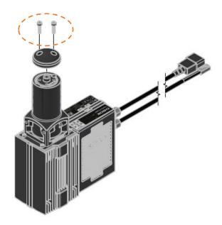
STEP 2: Attach the piston adaptor with the four (4) provided screws. Apply some blue thread locker on the screw threads then torque them to a value of 100 lbf·in (11 Nm) using a 4mm Allen Key:
